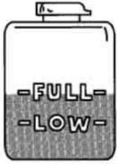
Fig.6.4. Reserve tank coolant level
