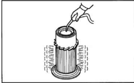
Fig.10.7. Cleaning air cleaner element
