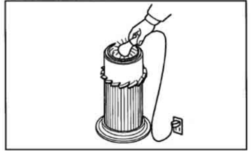
Fig.10.8. Checking air cleaner element
